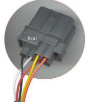
Fig 4. L1H1 Sensor 's Connector (Sumitomo)
