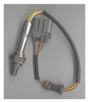
Fig 3. NTK L1H1 Wideband Sensor
